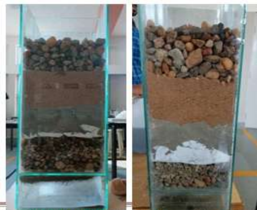
Figure 8: Filter Bed Figure 9: Filter Bed using Fly Ash using Wood Ash
